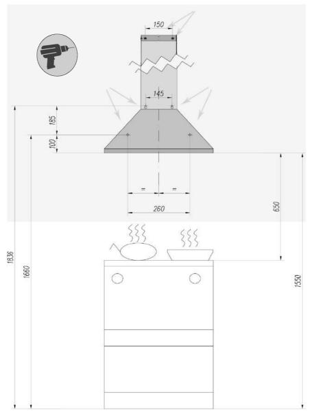
HOOD MUST BE INSTALLED ON MINIMUM 5" DUCTING OR RECTANGULAR EQUIVALENT
